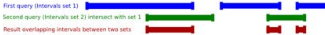
Figure 1.1: Graphical example of intersections between two sets of intervals which has to be detected by unioionBed program.
