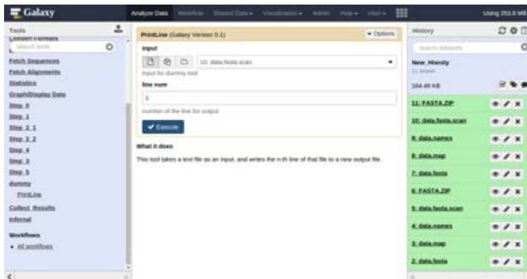
Figure 3.3: Integrated PrintLine Tool. All tools integrated in Galaxy have a uniform graphical interface.
