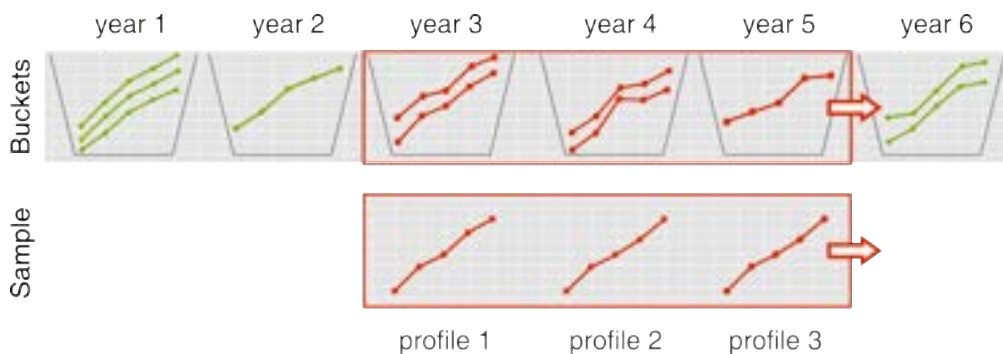
Figure 3.5.1.1 Schematic profile-wise shifting. A sample of length 3 is shifted along a Buckets Chronology of length 6. To compute a distance for a specific start-year, every sample profile is compared with each profile from the corresponding bucket.
