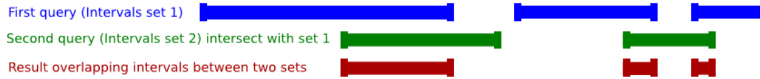
Figure 1.1: Graphical example of intersections between two sets of intervals which has to be detected by unionBed program.
